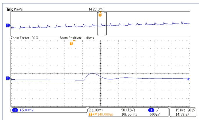
**Figure 12.** This scope capture shows a portion of the current measurement from a cyclic voltammogram of potassium ferrocyanide generated with a scan rate of 100mV/s. In the enlargement, the significant charge transferred through the cell, from the step can be clearly delineated. The analog integration method uses all this transferred charge in the current calculation at each step of the C-V plot.
