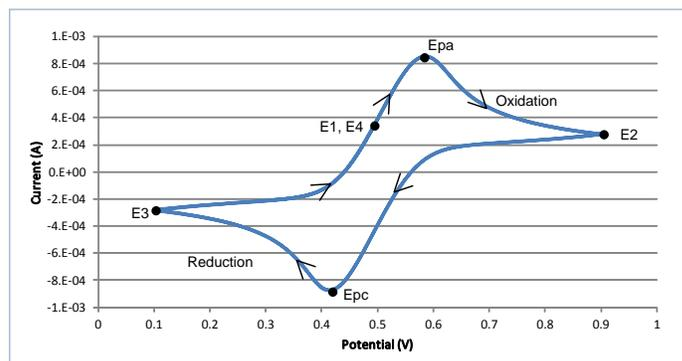
Figure 3. Example voltammogram generated using Model 2450-EC system.
