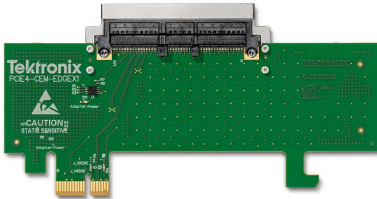
Figure 1: PCIe 4.0 x1 CEM Edge adapter
