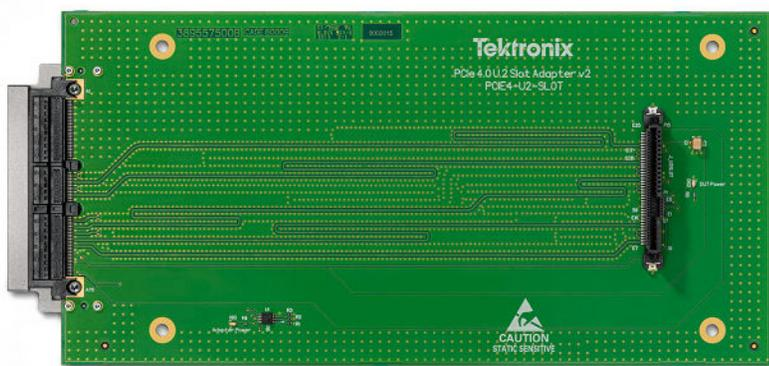
Figure 10: PCIe 4.0 U.2 Slot adapter
