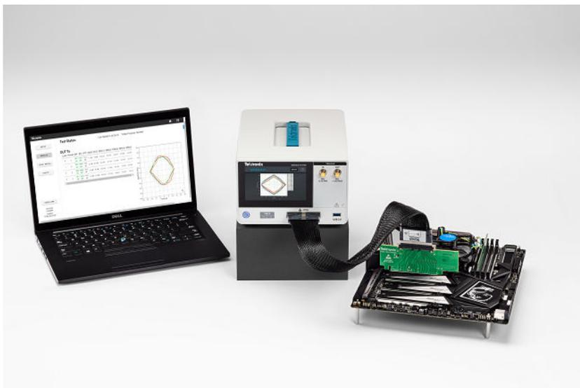
Figure 13: Quick scan setup example using a x16 CEM Edge adapter for motherboard testing. Quick scans can be run and results seen from the front panel and the web UI.
