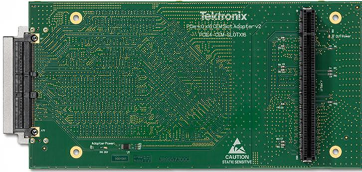
Figure 5: PCIe 4.0 x16 CEM Slot adapter
