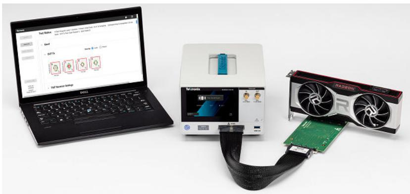
Figure 14: Custom scan setup example using a x16 CEM Slot adapter for graphics card testing. Custom scan can only be run and results seen from the web UI.
