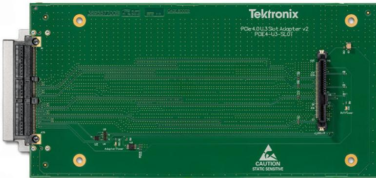
Figure 12: PCIe 4.0 U.3 Slot adapter
