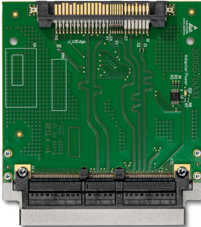
Figure 11: PCIe 4.0 U.3 Edge adapter
