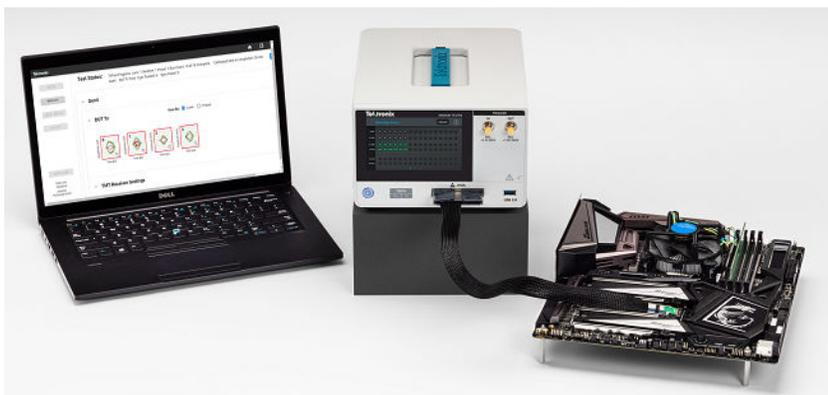
Figure 15: Setup using M.2 Edge adapter and integrated cable for motherboard testing.
