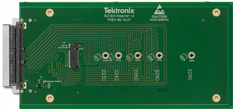
Figure 8: PCIe 4.0 M.2 22mm Slot adapter
